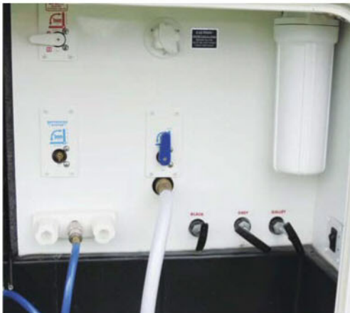
(right) From top left and going clockwise: hot-water valve, black-tank flush, water filter, tank-dumping handles, fresh water inlet, outdoor faucet/hose and winterizing system.
